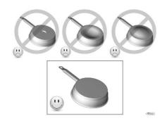
Cookware with a curved base or indentations on the base can cause permanent damage to the hob and lead to the failure of electronic components.
